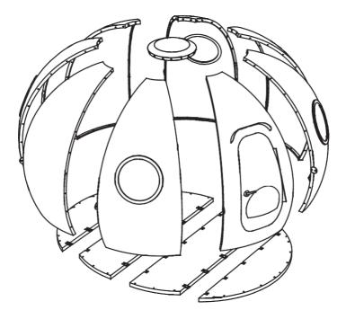
The basic Igloo Satellite Cabin consists of three plain panels, four window panels, one door panel with rain hood, one topknot and four floor panels. Wall panels may be purchased separately to create the configuration best suited to your needs e.g. seven window panels and one door panel for all round observation, or seven plain panels and one door panel for a photographic darkroom.
