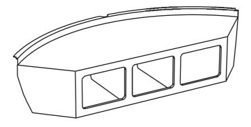
Each bunk 500mm high, 770mm wide and fits within the curved width of two wall panels, enabling three bunks to fit within the basic Cabin. Two bunks can be fitted one on top of the other to provide extra storage space with a large shelf area.
