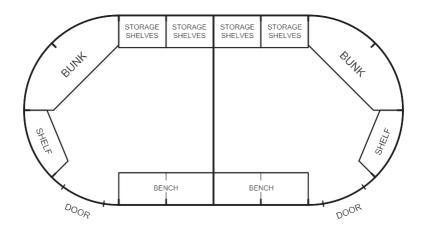
This four-section extended Cabin has two doors, which allow the Cabin to be divided by a partition. Though the Cabin is shown with only one bunk at each end, a two-section straight bunk can be set up each side of the partition to double the number of occupants.
