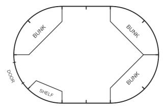
By extending the basic Cabin with two sets of extension panels, 1500mm additional space is provided for workspace and storage. Total length is 4500mm.
