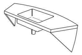
This is a standard shelf unit with a sink moulded into it. The sink is suitable for kitchen or laboratory use and can be fitted with a straight hose to bucket or with an "S" trap to empty through the side wall of the Cabin. An outlet plug is included with the unit.
