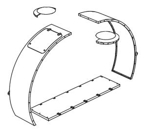
Each set of extensions add 765mm to the length of a Cabin and includes one wall panel with an escape hatch, one plain panel, two half top-knots with an air vent in each, and a floor panel. Added sets of plain wall panels and floor panels make up the required length.
