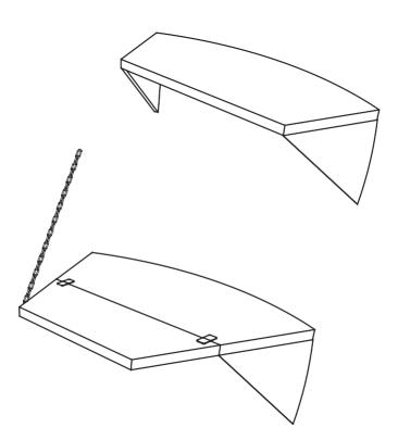
Each shelf fits the curved width of a wall panel and is 450mm deep. The desk is a shelf with a 308mm hinged flap, supported by a chain. Up to seven shelves or desks can be fitted within a basic Cabin.
