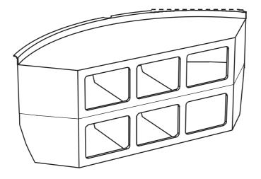
This double workbench spans two panels of a basic Igloo Satellite Cabin and provides a large surface for all bench work. There are 6 divided storage areas. The back of the bench top has a lip to stop small items rolling off it.
