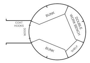
Where wet conditions prevail, the entrance tunnel will protect the inside of the Cabin from driving rain. There is enough space within the entrance for hanging wet clothes and storing boots. In addition to two bunks and a shelf, a double workbench can be added to provide extra storage as well as a large working surface. The double workbench can be used as a bunk if necessary.
