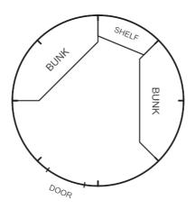
This basic Cabin contains only two bunks and one shelf, leaving space to add an extra bunk at a later date if required. For transport, the complete Cabin and contents can be lifted by helicopter and flown at up to 70 knots.
