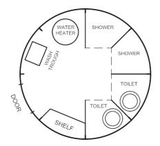
The above drawing shows one type of layout for the Igloo Satellite Cabin as a sanitary unit.
