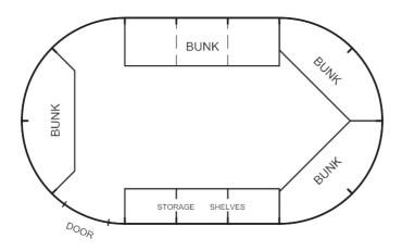
Adding three sets of extension panels to the basic Cabin provides enough room to add a three-section straight bunk. A second bunk may be added on the opposite wall.
