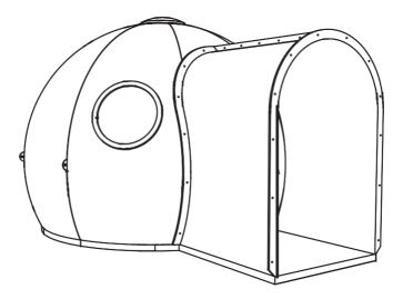
Each entrance tunnel is 1200mm long and is wide enough to allow the door to open fully. Coat hooks can be installed on the innersides of the tunnel to allow wet clothing to dry, or to shelter stores. Tunnels can be attached by bolts to Cabins and attached to each other to interlink Cabins.
