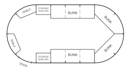
This Cabin with four sets of extension panels is 6000mm long and is shown with bunks for four people. However, an extra bunk may be added at the door end to enable the Cabin to sleep five.
