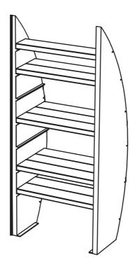
The shelves of this unit fit within the width of an extension panel and can be set on to seven different levels to accept a large range of items. Each shelf unit can be assembled side by side along one side of an extended Cabin or set opposite each other to provide a partial divider inside a Cabin.
