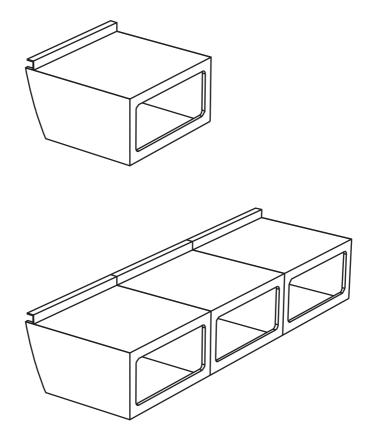
Each seat fits within the width of an extension panel. These seats can be bolted together to form a straight bunk with a total length of 2300mm and width of 700mm.
